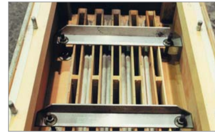
Fig. 2b: Bag air filter (compressor side)
