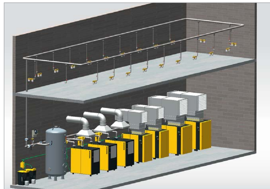
Example of a compressed air station with exhaust air system and thermostatically controlled additional ventilation for the refrigeration dryers
