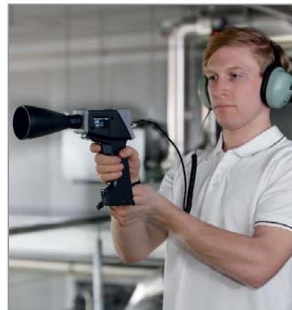
Fig. 4: Leakage location using ultrasound
